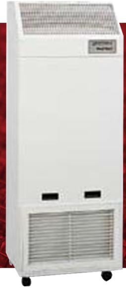
**This portable, self-contained high-efficiency particulate air (HEPA) filtration system is designed to easily and economically create a negative pressure isolation room/environment that will meet OSHA and CDC TB guidelines.**
